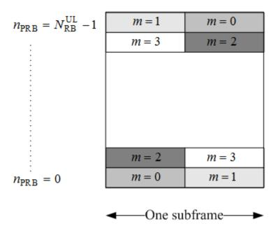
PUCCH formats 1, 1a, and 1b make use of four SC-FDMA symbols per slot. If normal cyclic prefix is used, the remaining 3 symbols, 2 for extended cyclic prefix, are used for PUCCH demodulation reference signal (DRS). If the sounding reference signal (SRS) overlaps the PUCCH symbols, only three symbols are used in the second slot of the subframe. The mapping of the symbols is illustrated in the following figure.
