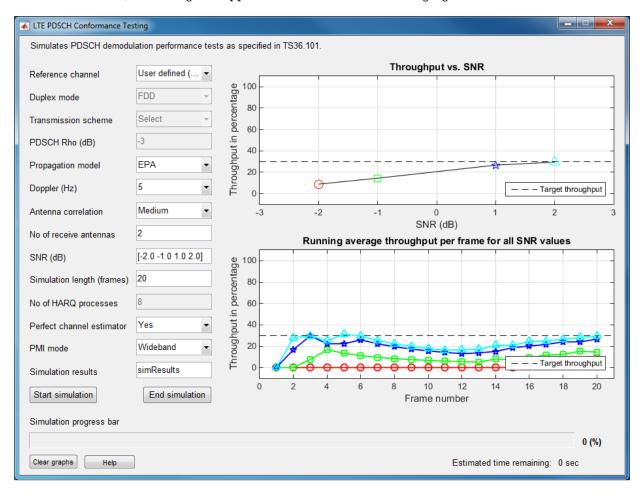
The simulation result for a 20-frame run is displayed in the MATLAB Command Window.
