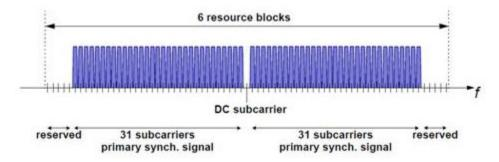
As the DC subcarrier contains no information in LTE this corresponds to mapping onto the middle 62 subcarriers within an OFDM symbol in a resource grid. d(n) is mapped from lowest subcarrier to highest subcarrier. The PSS is mapped to different OFDM symbols depending on which frame type is used. Frame type 1 is frequency division duplex (FDD), and frame type 2 is time division duplex (TDD).
