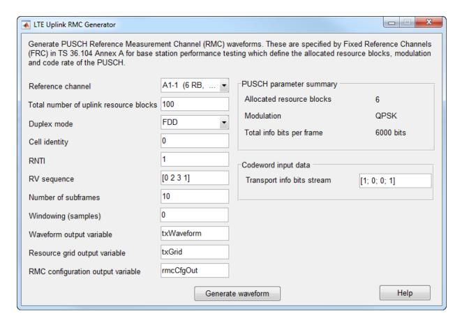
Click the **Generate waveform** button. The variables txWaveform, txGrid, and rmcCfgOut now appear in the MATLAB Workspace Browser.
