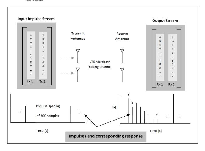
Pre-configure the LTE multipath fading channel. To do so, set up a simple structure and specify the fading channel parameters.
