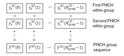
The variable  $y_i^{(p)}(n)$  is the *n*-th element within PHICH *i* on antenna port *p*.
