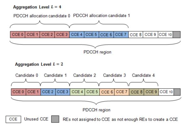
In this example, only 11 CCEs are available due to bandwidth constraints. The CCEs used to construct each PDCCH candidate are defined by the following equation.
