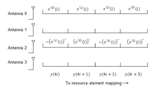
If  $n_{PHICH}^{group} + i$  is odd for a normal cyclic prefix or if  $\lfloor n_{PHICH}^{group}/2 \rfloor + i$  is odd for an extended cyclic prefix, the relationship between the input and output is defined by the following equation.
