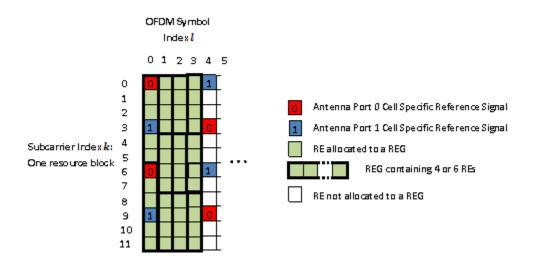
Cell-specific reference signals are present within the first OFDM symbol. As four REs not containing cell specific reference signals are required in a REG, the twelve REs in the first symbol are divided into two REGs, each containing six REs (two containing cell specific reference signals and four empty). In the second and third OFDM symbols no cell specific reference signal is present therefore the twelve REs in each symbol are divided between three REGs, each containing four REs.
