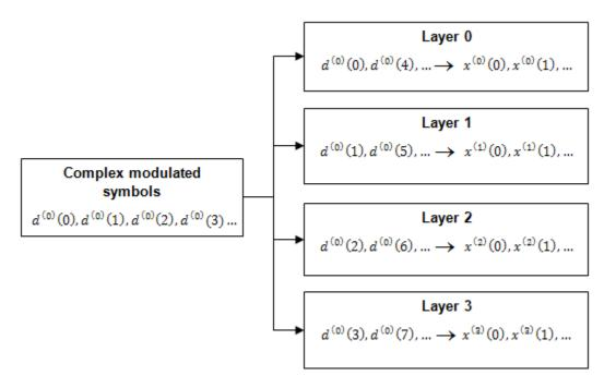
If the total number of input symbols is not an integer multiple of four  $(M_{symb}^{(0)} mod 4 \neq 0)$  two null symbols are appended onto the end. This creates a total number of symbols that is an integer multiple of four because the original number of symbols is always an integer multiple of two.
