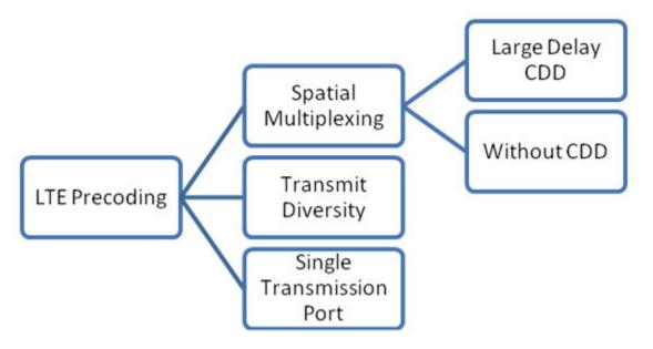
The precoder takes a block from the layer mapper,  $x^{(0)}(i), x^{(1)}(i), ..., x^{(v-1)}(i)$ , and generates a sequence for each antenna port,  $y^{(p)}(i)$ . The variable p is the transmit antenna port number, and can assume values of  $\{0\}, \{0,1\}, \text{ or } \{0,1,2,3\}$ .
