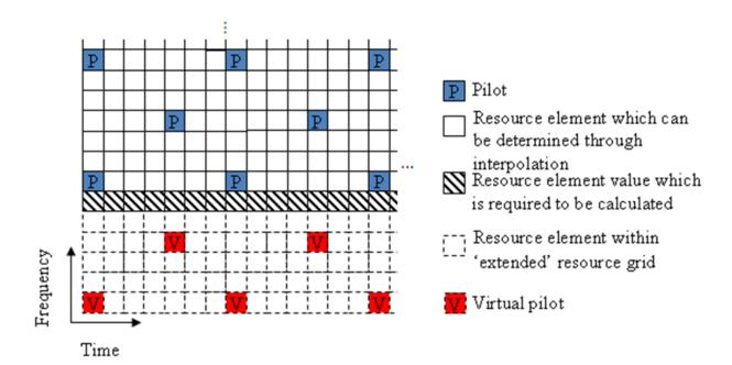
In this system, the resource grid is extended, with virtual pilot symbols created in locations which follow the original reference signal pattern. The presence of virtual pilot symbols allows the channel estimate at the resource elements, which previously could not be calculated by interpolation, to be calculated by interpolation using the original and virtual pilot symbols.
