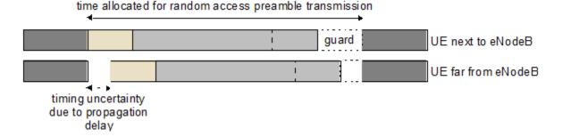
Therefore the size of the guard period determines the cell radius, as any propagation delay exceeding the guard time would cause the random access preamble to overlap the following subframe at the eNodeB receiver.
