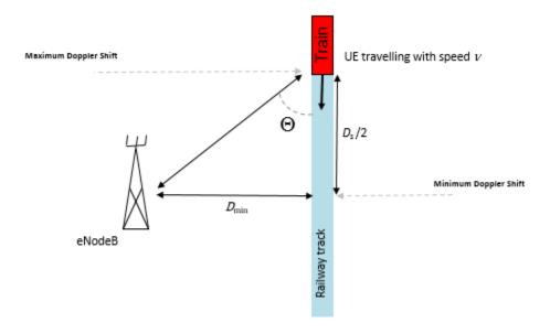
The expression  $D_s/2$  is the initial distance of the train from eNodeB, and  $D_{\min}$  is the minimum distance between eNodeB and the railway track. Both variables are measured in meters. The variable  $\nu$  is the velocity of the train in meters per second. The Doppler shift due to a moving train is given in the following equation.
