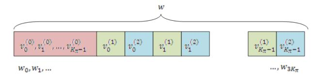
Interlacing allows equal levels of protection for each parity sequence.
