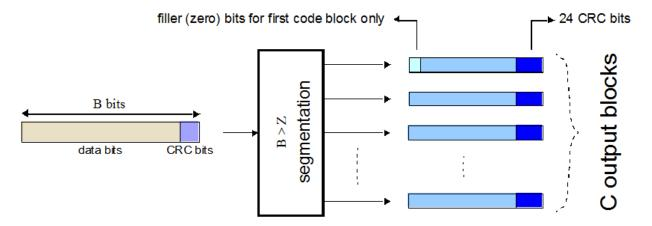
If no segmentation is needed, only one code block is produced. If *B* is less than the minimum size, filler bits (zeros) are added to the beginning of the code block to achieve a total of 40 bits.
