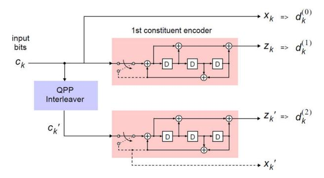
The output of the encoder is three streams,  $d_k^{(0)}$ ,  $d_k^{(1)}$ , and  $d_k^{(2)}$ , to achieve a code rate of 1/3.
