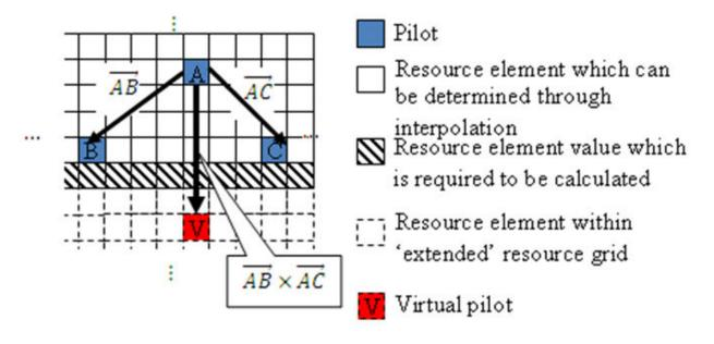
**Note** Virtual pilots are only created for the MATLAB® 'linear' and 'cubic' interpolation methods.
